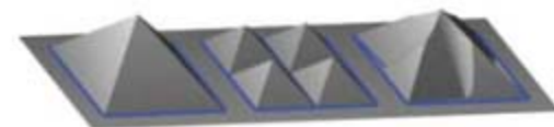
Fig. 2. (Left) A square road pattern produces a pyramid of roadless volume. (Center) Four added roads, each of length = 0.5 \times (the length of one pyramid side) and intersecting at the center (the two roads parallel to the long side of the image are mostly hidden), reduce the pyramid volume by 50%. (Right) Four roads of the same length, starting at the corners and angled slightly toward the center (tan divergence angle = 0.1), diminish the pyramid volume by only 13.5%.
